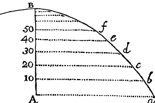
2d. Make the lines  $Aa$ ,  $10b$ ,  $20c$ ,  $30d$ ,  $40e$ , &c. respectively equal to the chords of  $90^\circ$ ,  $80^\circ$ ,  $70^\circ$ ,  $60^\circ$ ,  $50^\circ$ , &c. to the radius AB, and the points  $a$ ,  $b$ ,  $c$ ,  $d$ ,  $e$ , &c. will be in the curve of the parabola.
