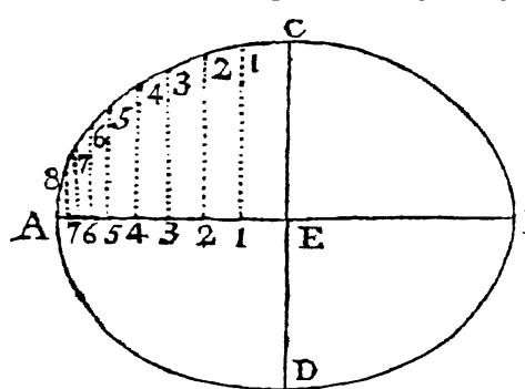
SOLUTION. 1st. Set the two diameters AB, CD, at right angles to each other in their middles at E.
